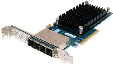
ATTO ExpressSAS® 12Gb/s SAS GT Model host bus adapters (HBAs) provide high-performance direct attach connectivity for server storage, JBOD and RAID arrays.
